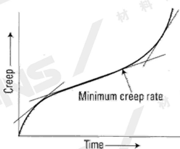
**Creep Limit**—Alternate term for Creep Strength.
