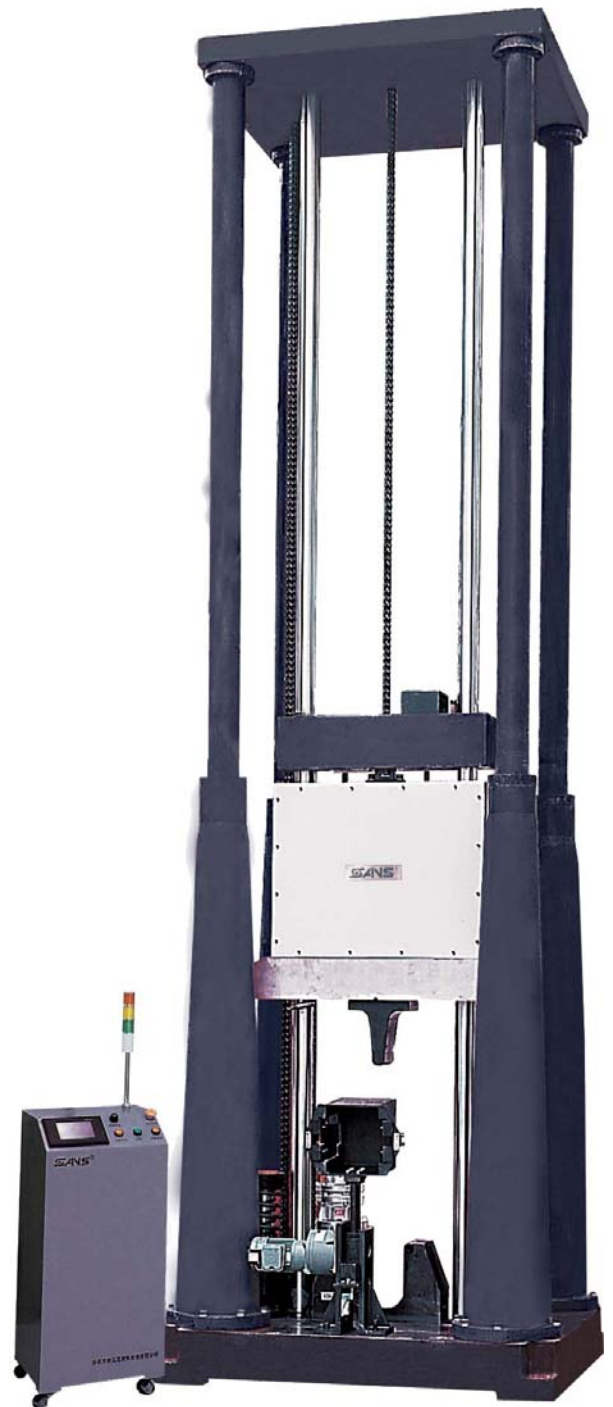
Fig2. ZCJ2304 (DWTT test)
