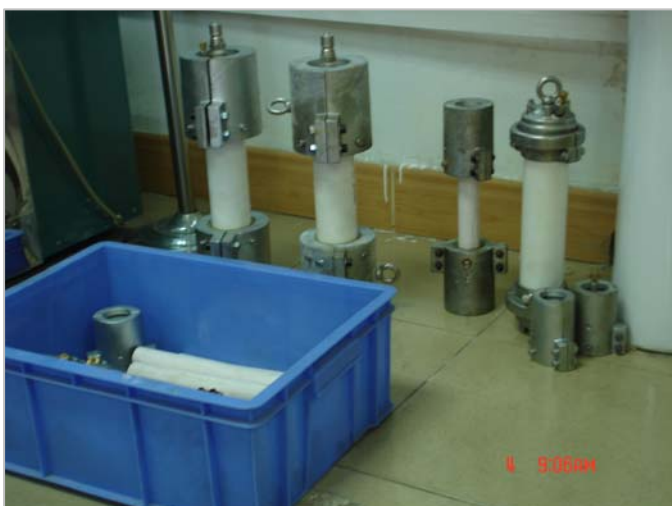
Fig5. Specimens and grips ready for test
