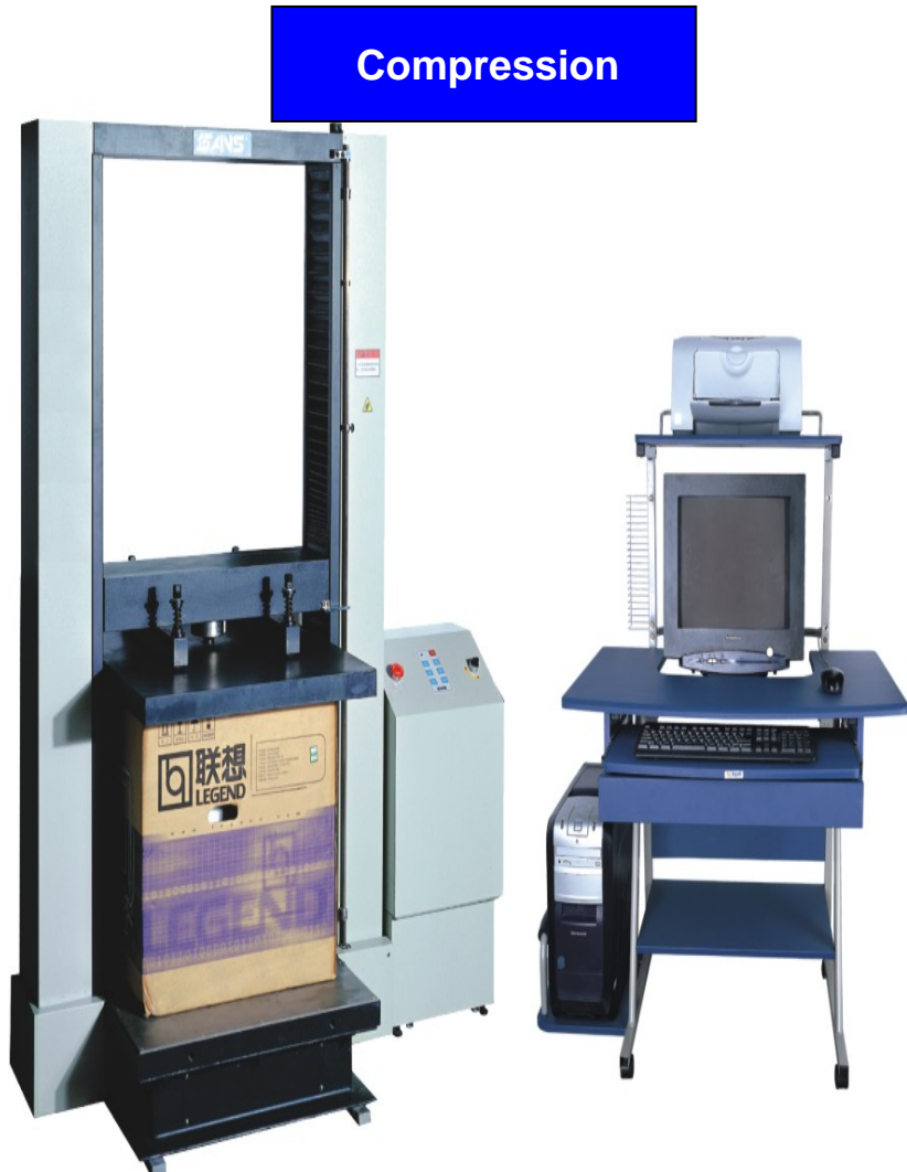
Fig1 CPT Series Packaging Container Compression Testing Machine
