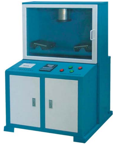
Fig3. ZQD series window/door corner strength testing machine
