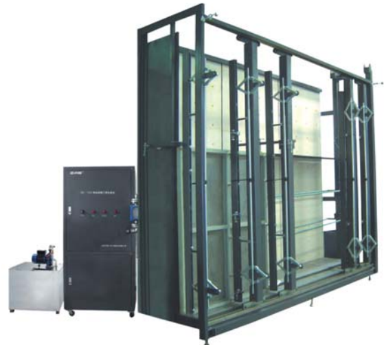
Fig1. ZMC series window/door Performance testing machine
