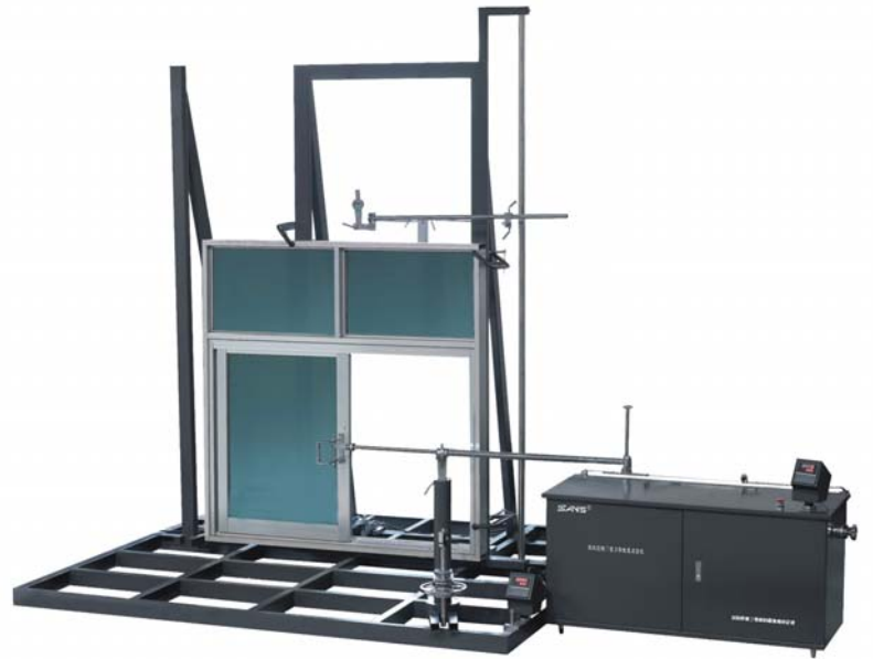
Fig2. ZML series window/door Mechanical testing machine
