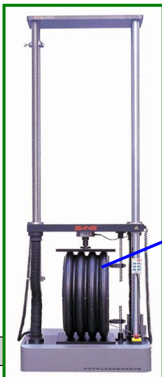
Fig2. RST304 used in ring stiffness testing
