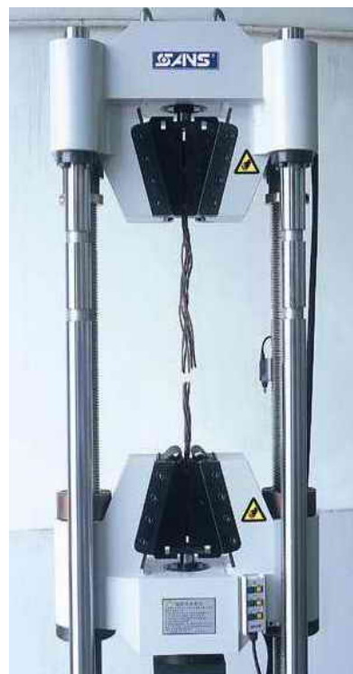
Tensile test of strand steel
