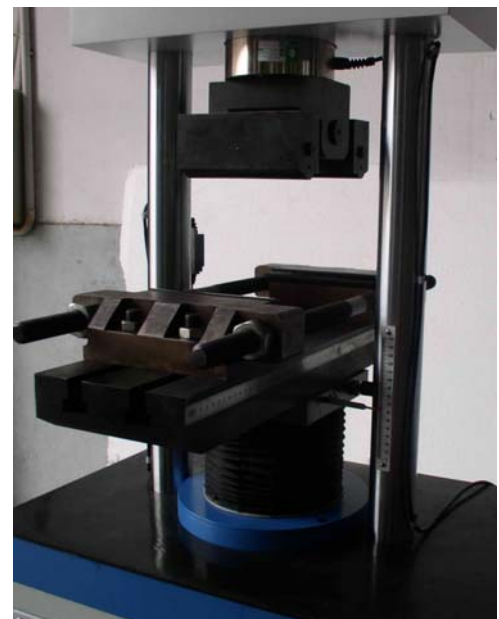
Fixtures for break-resistant test of cement
