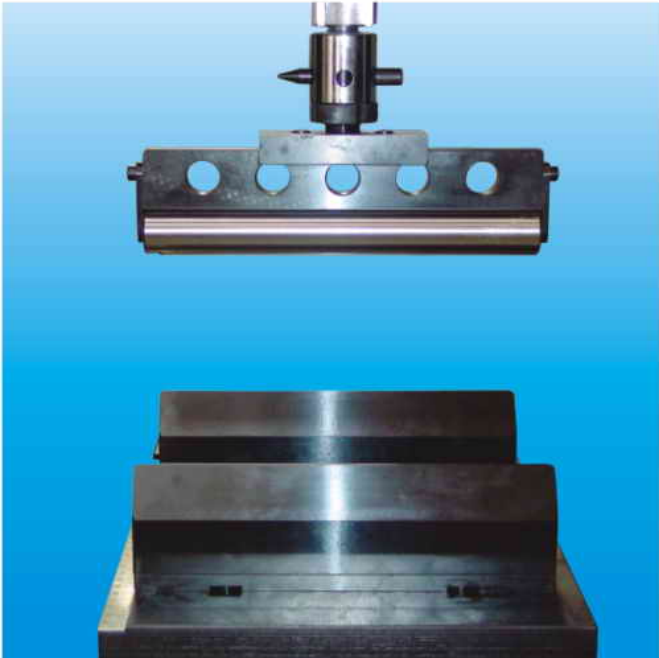
Fixtures for break-resistant test of bricks
